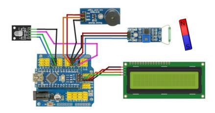
The reed switch is connected to digital pin 4 of Arduino board. The 1602 LCD is connected to the I2C interface. The passive buzzer module is connected to digital pin 5 of Arduino board. The R (red) pin, G (green), B (blue) pin of the RGB LED module are connected to digital pin 3, 10, 11 respectively. Do notice that not all digital pins have PWM. The PWM function only works on pins 3, 5, 6, 9, 10, and 11 of Arduino NANO
