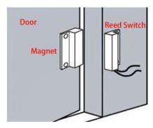
A door alarm system would usually consist of a reed switch, a sounding device and a lighting device. Normally, high decibel buzzers and special flashing signal lights would be used, but they are not very pleasant for practices at classroom or home.
