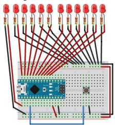
There are a total of twelve LEDs connecting to digital pin 2-13 of the Arduino board. There is a push button connecting to analog pin A0 of the Arduino board. The analog pin A0 is also called digital pin 14.
