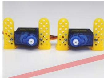
Then, install the two servo motors on the perforated plastic panel midway on the left and right sides with 6mm M3 sharp screws applied to their attached perforated angle brackets. Ensure that both servo motors' output shafts are aligned (on the red line shown in the figure) and positioned closer to the front end. When done, pass the wires of the servo motors through the rectangular hole on the panel for later use.
