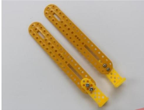
Next, install the four assembled sets of perforated strips and angle brackets to the four corners of the perforated plastic panels with 8mm M2 nuts and bolts applied to the perforated angle brackets in the corners. Given that flexible joints would enable smooth movement for the Hexabot, ensure that the nuts and bolts are not applied too tightly between the strips and the angle brackets in the corners. Allow some room for the strips to swivel.
